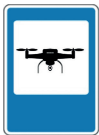
■ Figure 1. The image of the proposed project of the information sign is numbered “5.70.1. – photo and video recording of traffic violations from UAVs”
